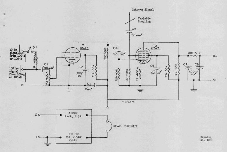
The above circuit will, when operated with a Model 100-A or 100-B, provide a method of frequency calibration up to 20 mc. With care, this mixer is usable up to 30 mc. The strength of the unknown and standard signals should be adjusted to give just a satisfactory signal in the headphones. Very strong signals will result in beats between sub-harmonics, obscuring the wanted check points.
